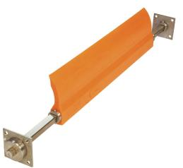
The <u>Martin® Compact Cleaner</u> from Martin Engineering uses a low-profile blade mounted on an internal square mainframe for effective belt cleaning in tight spaces. It is designed for applications on small pulleys and belts operating at speeds up to 350 fpm (1.78 m/sec).
